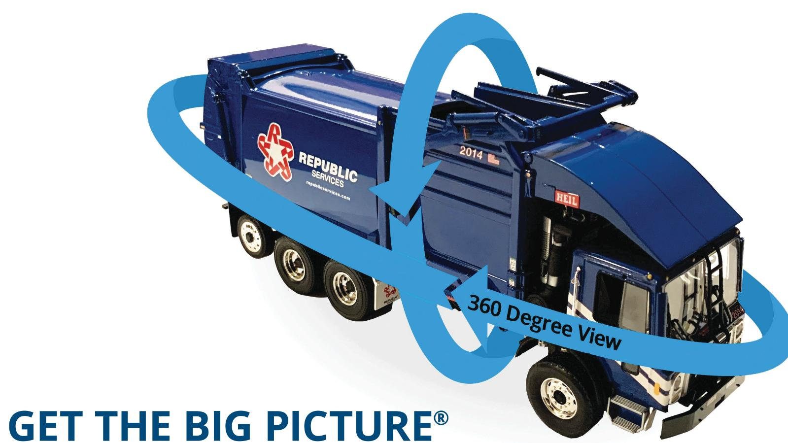
Complete a Full Scan every 5 to 8 Seconds to establish a circle of safety around the truck (360-degree view)
